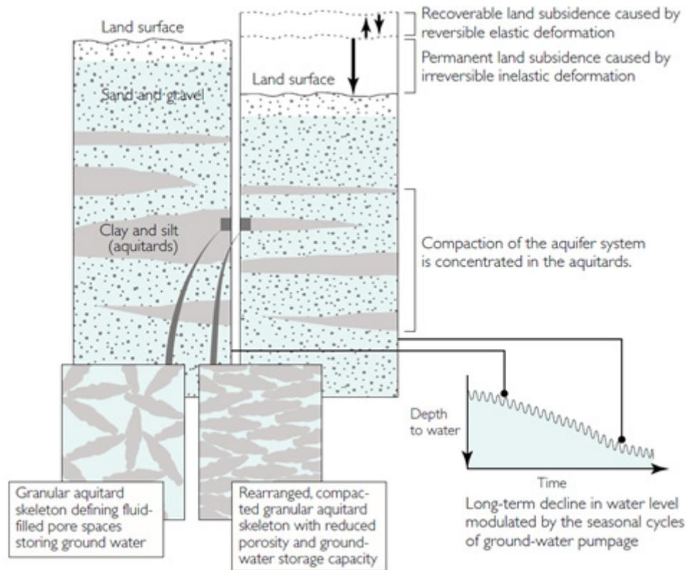
Figure 1 Subsidence from groundwater withdrawal and depressurisation.
